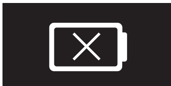
Low Battery Indicator - Indicates the Handheld Control Unit will power off in 5 seconds and new batteries should be inserted into the device.
